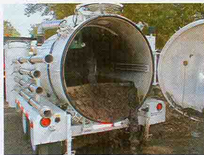
Pumper truck containing sediment sludge pumped from the swirl chamber.
